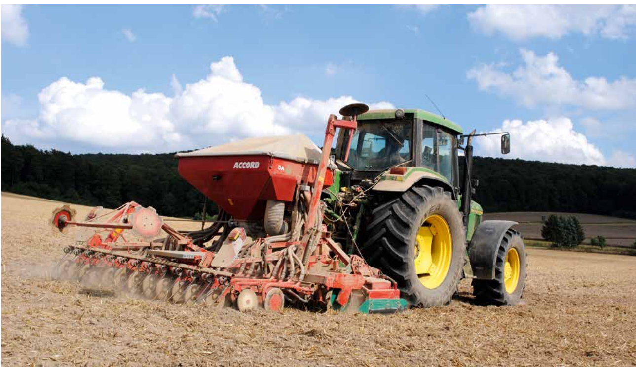
The use of the drill in a mulch bed provides preliminary protection of the soil surface against erosion and drying out.
