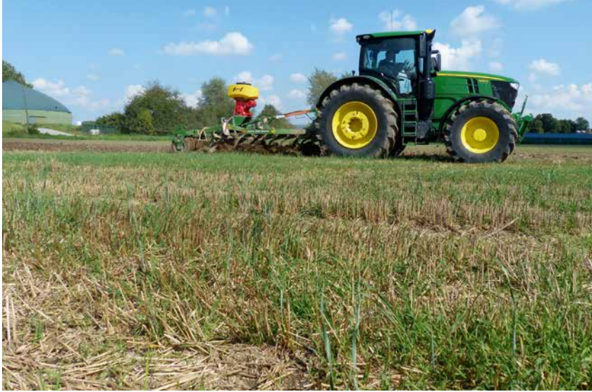
A pneumatic spreader on the soil tillage implement allows two operations to be combined.
